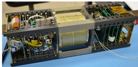
Figure 7. NRL TEPCE CubeSat with EDDE Components
