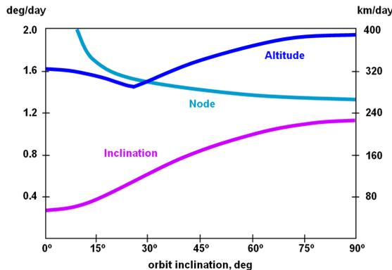
**Figure 3. 80 kg EDDE Orbit Transfer Rates per Ampere Average Current**
