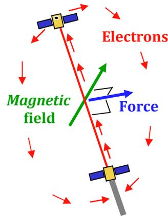
Figure 1. Electrodynamic Propulsion Concept
