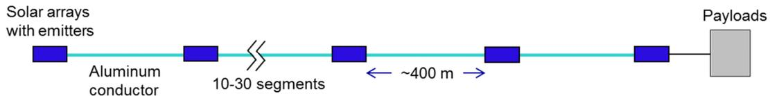
**Figure 2: EDDE Vehicle Schematic, Showing Arrays, Conductor, Emitters, and Payloads**
