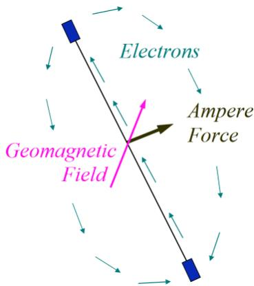
**Figure 2: Propellantless Propulsion**
