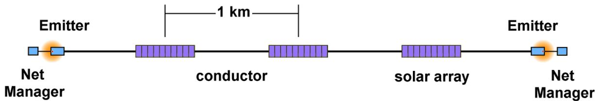
**Figure 3: Representative Sections of the 10-km-Long EDDE Vehicle**
