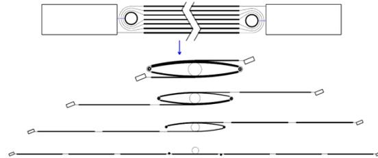
**Figure 5. Deployment of Laminated-film Solar Array**
