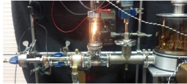
**Figure 8. Vacuum Testing of Thermionic Emitters**
