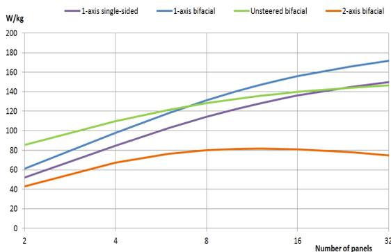
**Figure 6. Comparison of Average W/kg for Candidate Solar Arrays and Steering Options**
