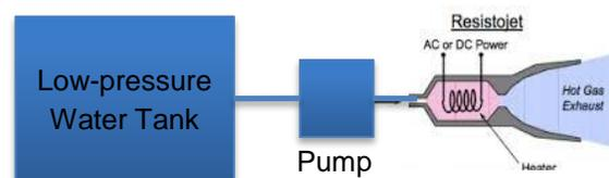
**Figure 11. Concept for 10-100 W Steam Resistojet**
