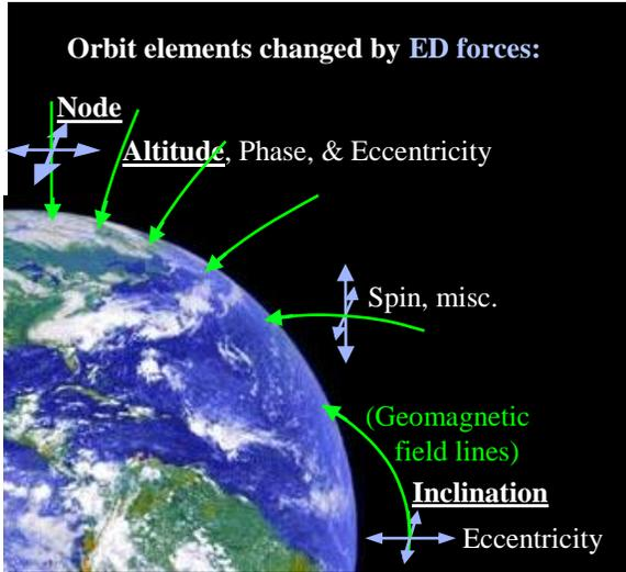
**Figure 3: Possible ED Thrust Vectors vs. Latitude**
