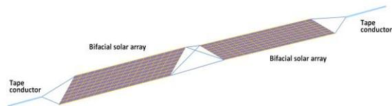
**Figure 7. Sub-Arrays Rigged to Stay at Right Angles**
