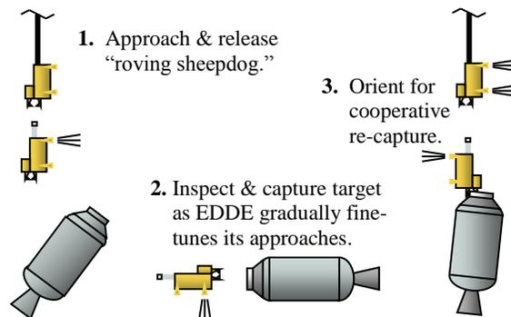
**Figure 18. "Two Dog Capture" of Passive Objects**
