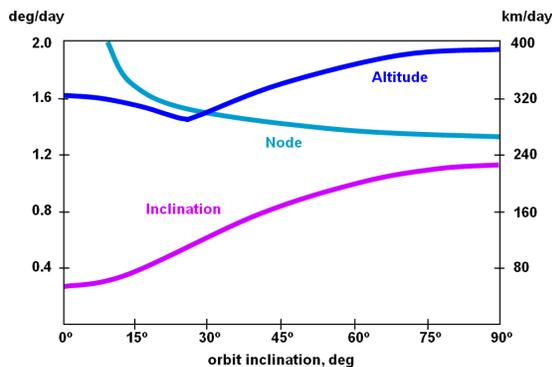
**Figure 4 EDDE Orbit Transfer Performance per Ampere Average Current, for an 80 kg EDDE**
