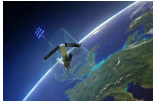
Figure 29. Thrown-Net Capture of Dead Satellite
