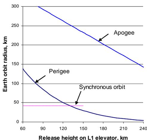
**Figure 9. Earth Orbit after Release**
