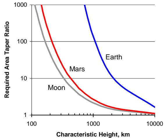
Figure 6. Space Elevator Taper Ratios
