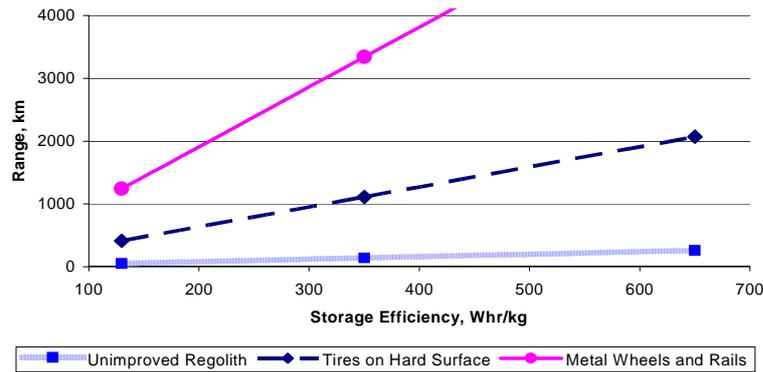
**Figure 14. Surface Vehicle Range vs. Storage Efficiency**
