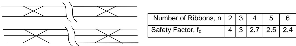
**Figure 7. Fail-Safe Ribbon Design**
