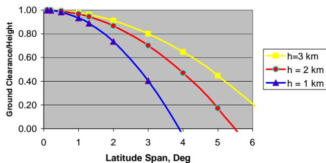
**Figure 11. Tower Span vs. Height**
