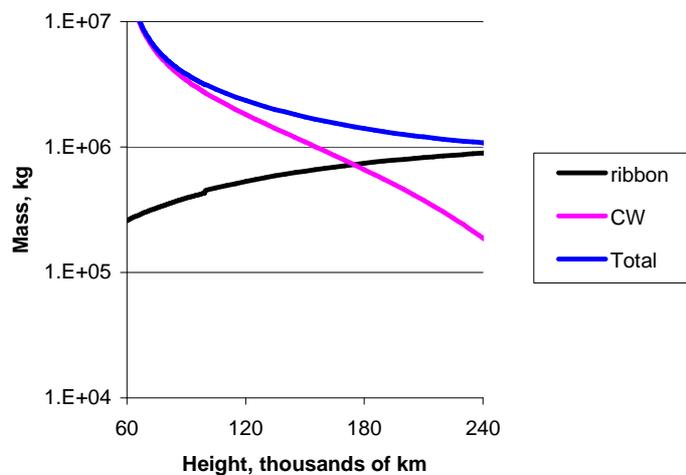
**Figure 8. Mass of the LSE Ribbon and Counterweight for Different Lengths**
