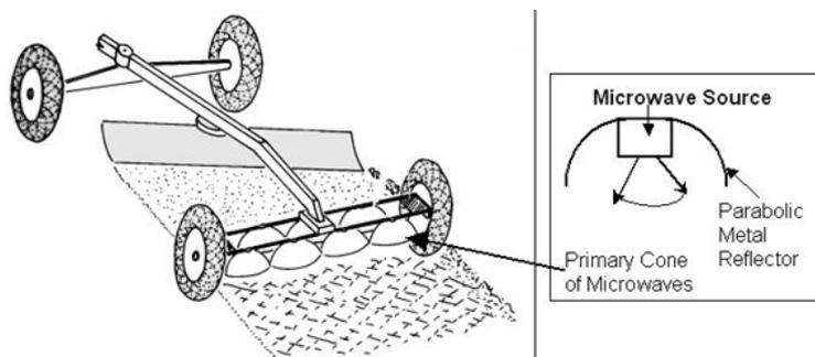
**Figure 13. Lunar Microwave Paving Machine**
