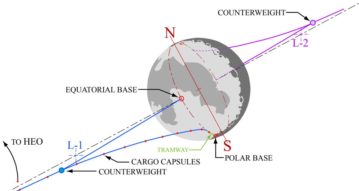
Figure 4: Lunar space elevators about L1 and L2, with equatorial and polar bases
