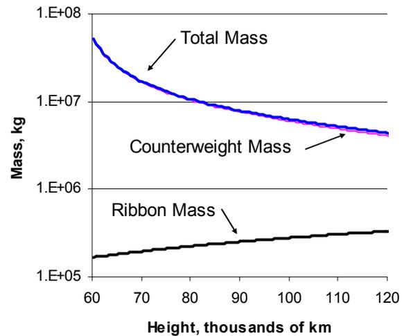
Figure 4: Lunar space elevator ribbon and counterweight mass
