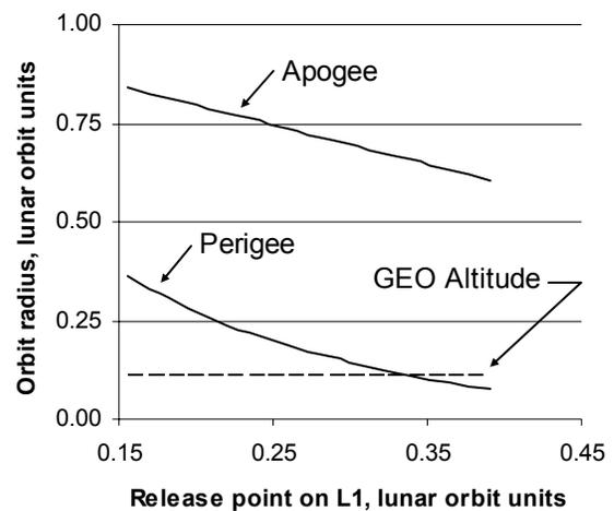
Figure 7: High Earth orbits reached by payloads from the L1 lunar space elevator
