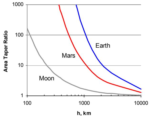
Figure 3: Space elevator area taper ratios vs. breaking height for Earth, Mars, and the moon
