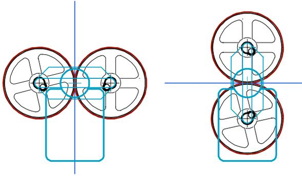
Figure 5: Climbing vehicles grip the ribbon, vertically or horizontally
